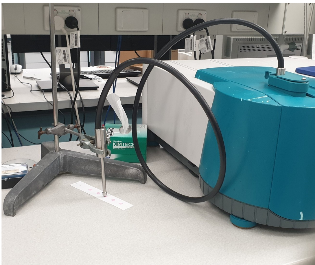
Figure 2.3: Experimental setup using the fibre optic probe for fluorescence measurements of amino acid spots treated with IND/Zn formulation containing different 1,2-indanedione concentrations.
