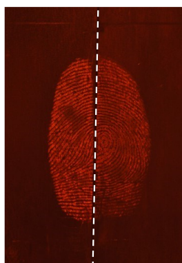
Figure 6.9: Comparison of cyanoacrylate fumed fingerprints stained by acid Nile blue for ten minutes (left half) and twenty minutes (right half), at 505 nm excitation wavelength of Polilight and viewed with 550 nm long-pass barrier filter.
