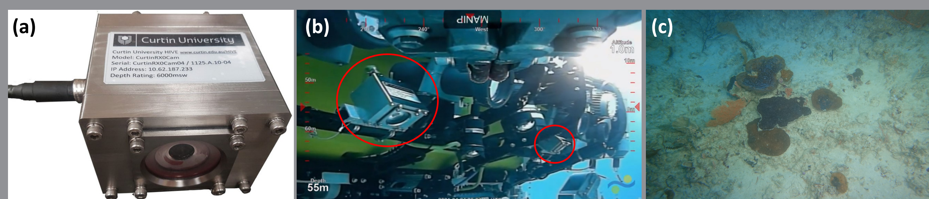
Figure 1. Still image capture: (a) CurtinRX0Cam-6000 camera, (b) as deployed on ROV SuBastian (seen inside the red circles), (c) example imagery from a mesophotic coral ecosystem at Ashmore Reef.
