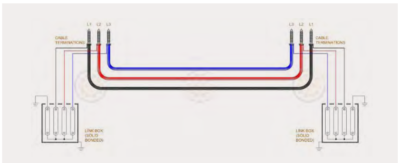
Figure 20. Solid Bonded Cable System (Electrotechnik 12 )
