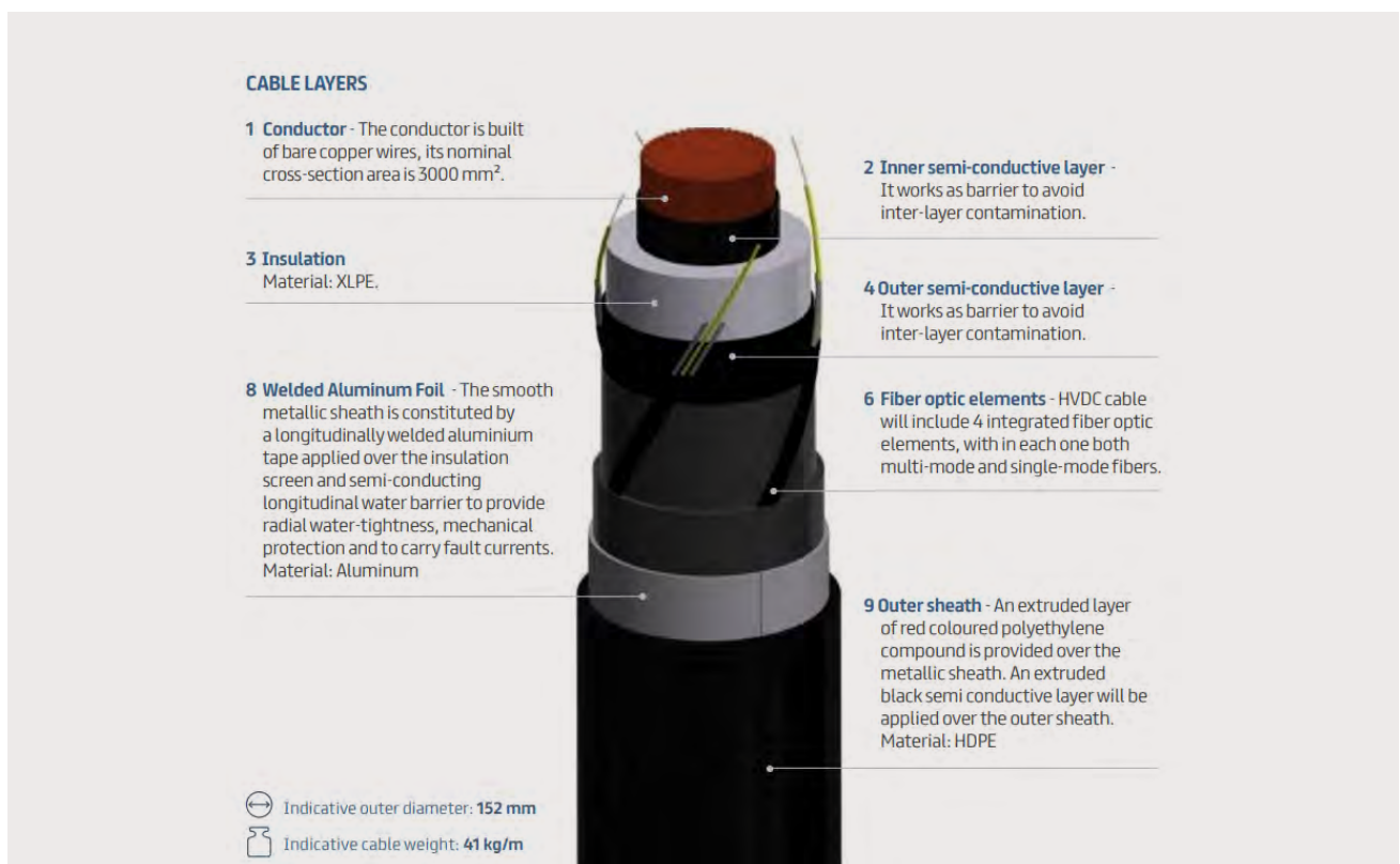
Figure 29. Suedlink HVDC XLPE Cable (Prysiam Group [26]).
