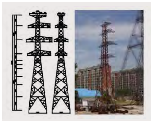
Figure 4 – General map of double circuits 110STJ tower [11]
