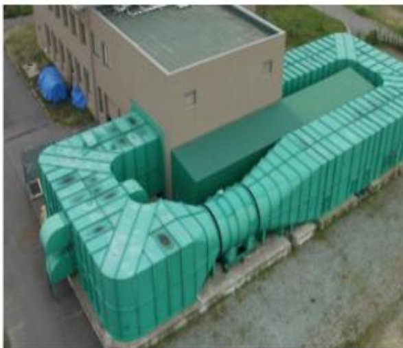
Fig 2.2. Wind tunnel by Li et al. (Li, Maeda, et al. 2016a, b)
