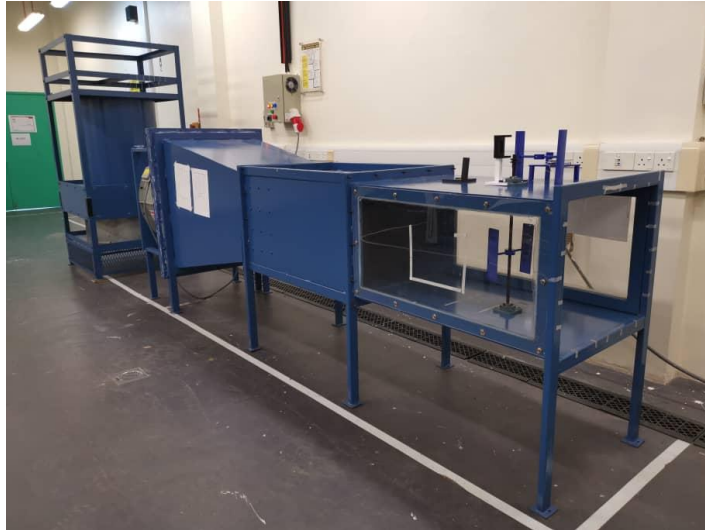
Fig 3.24. Wind tunnel used for experiments.
