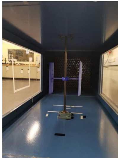
Fig 3.25. Test section area of the wind tunnel. Shown at back are the honeycomb design to straighten the flow.
