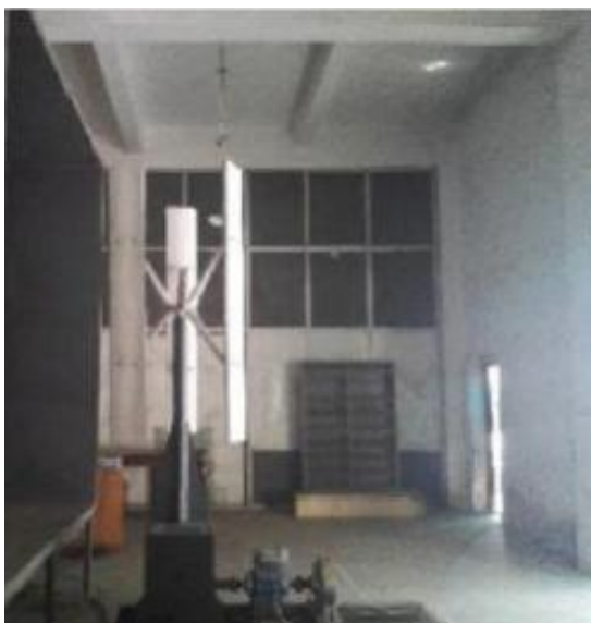
Fig 2.29. Two support-arm arrangement from He et al. (Hashem and Mohamed 2018).
