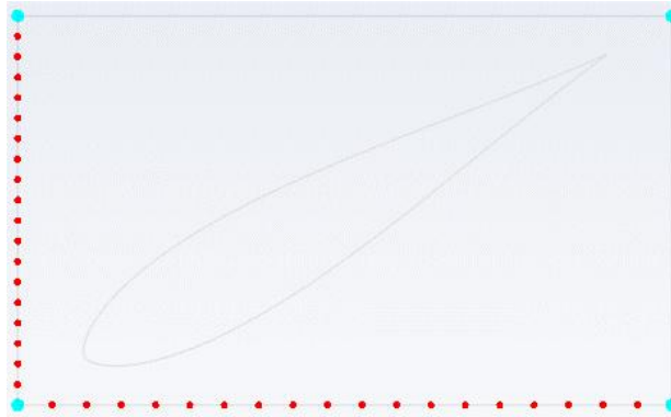
Fig 3.13. Bounding region and control points around the S1046 airfoil geometry set to 20 points each in the X and Y direction.
