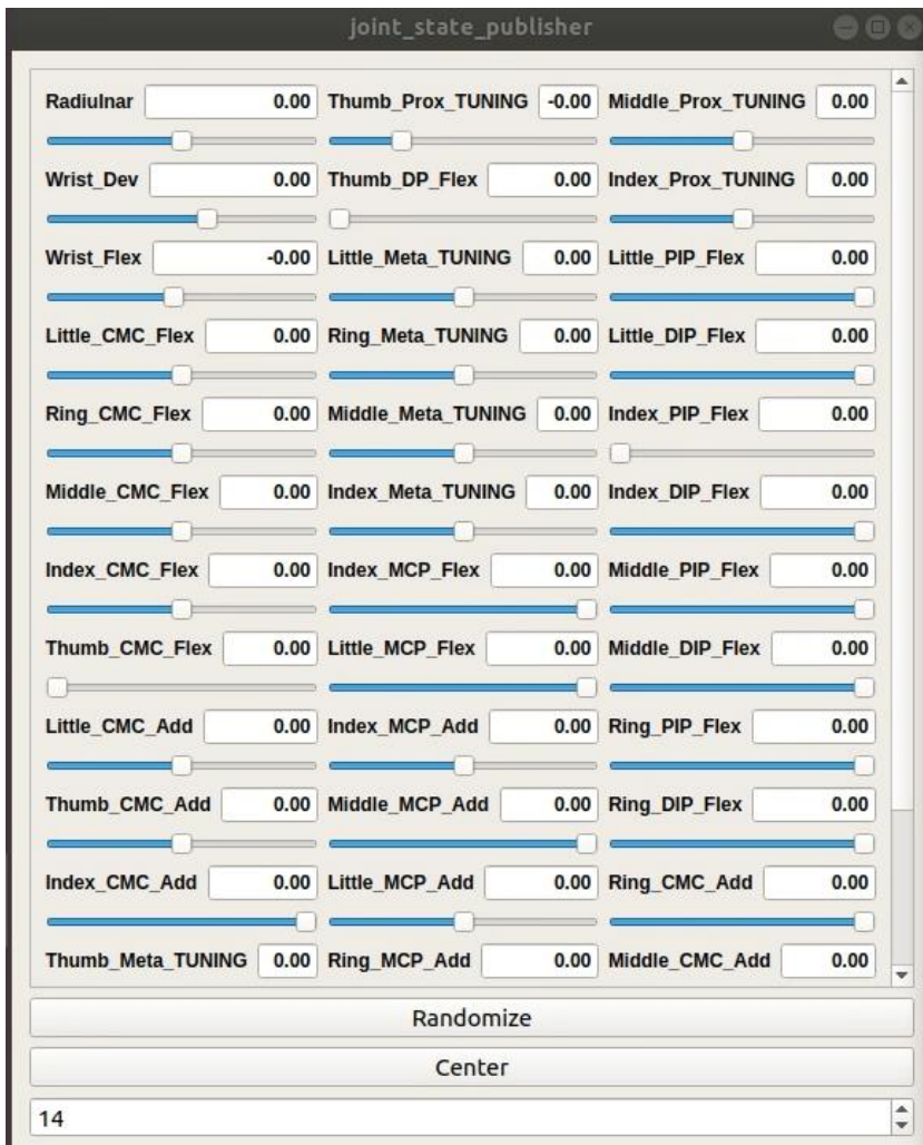
Figure 29 ROS RViz Hand Model full GUI. Contains both desired and tuning joint control.
