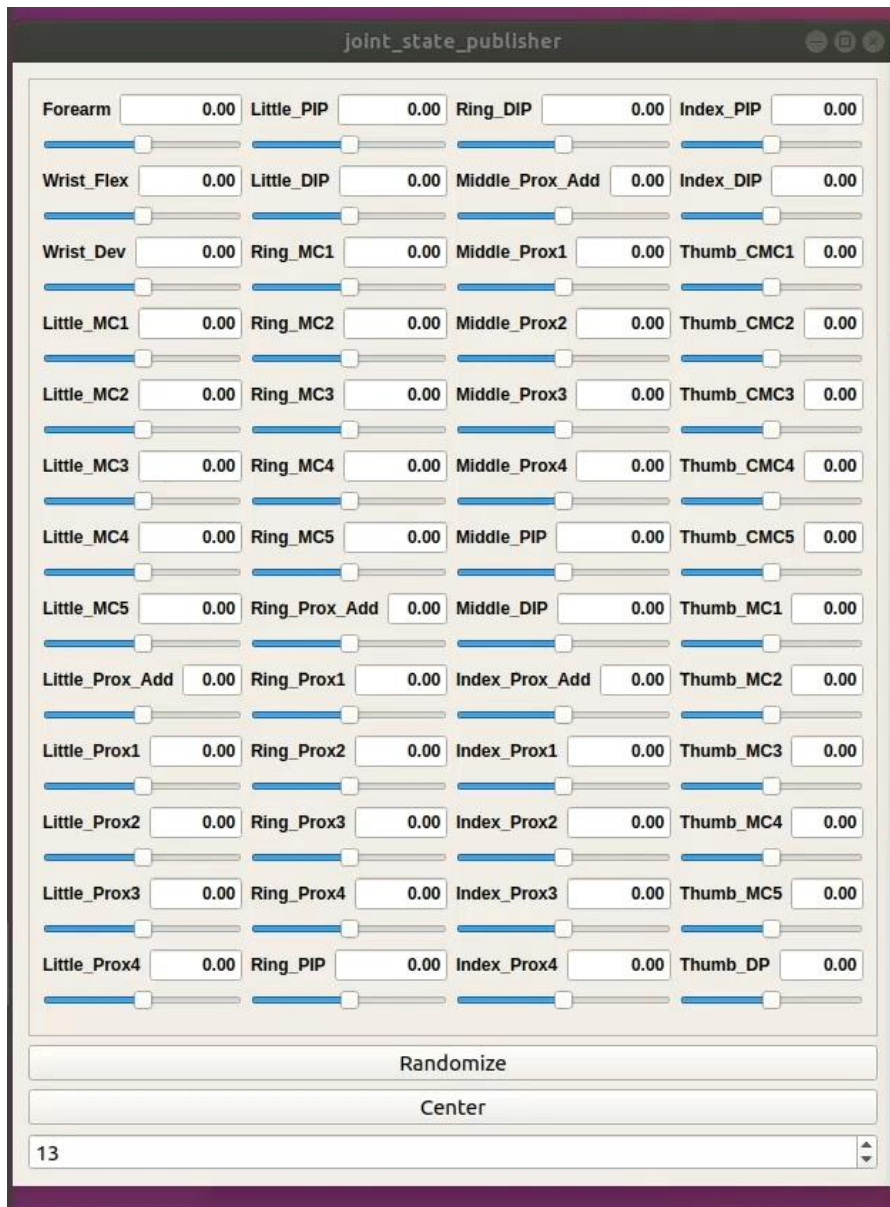
Figure 31 ROS RViz Orthosis Model full GUI. Contains desired, intermediate, and tuning joint control.
