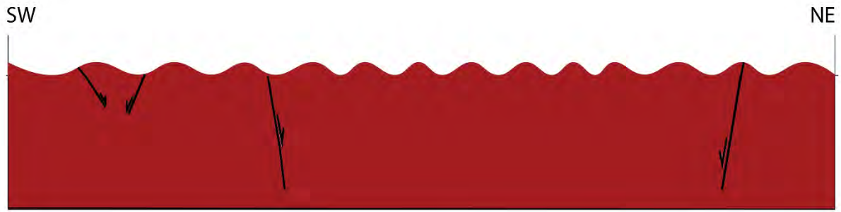
Figure 4-21a. Reconstruction of southwest-northeast Seismic composite line 1. The cartoon shows that the basement was assumed to be flat during pre-Paleogene.
