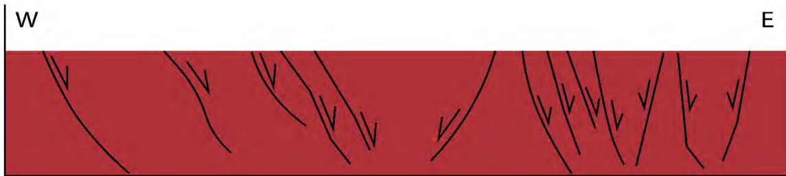
Figure 5-35a. Reconstruction of east-west Seismic line 255. The model show the initiation of rifting in the basement.
