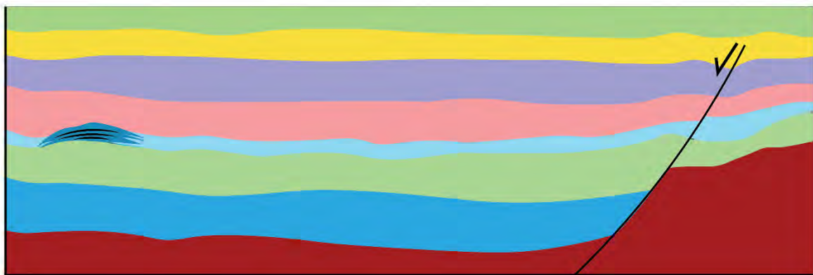
Figure 4-21 j. Inversion started during the deposition of Seurula fm during the Pliocene.
