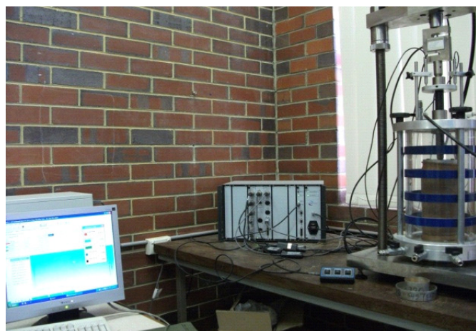
Figure 2. The UTM-14P digital servo control testing machine.
