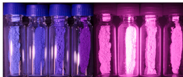
Fig. 3. EB-L, EB-K, HB, and HP respectively, pictured (left) under natural light ( f/22 , 1/125 s) and (right) under white light in NIR luminescence mode ( f/29 , 1.0 s, B & W IR lens filter).
