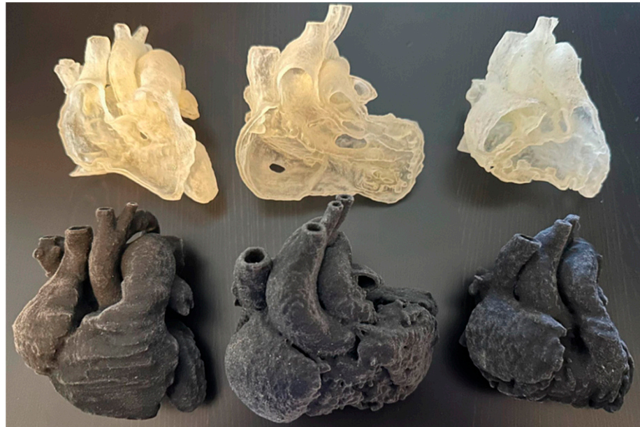
Figure 1. Models were printed with a flexible material, Agilus 30 (Objective 3D, Stratasys, Melbourne, VIC, Australia). VSD in the left column, DORV in the middle column, and ToF in the right column.
