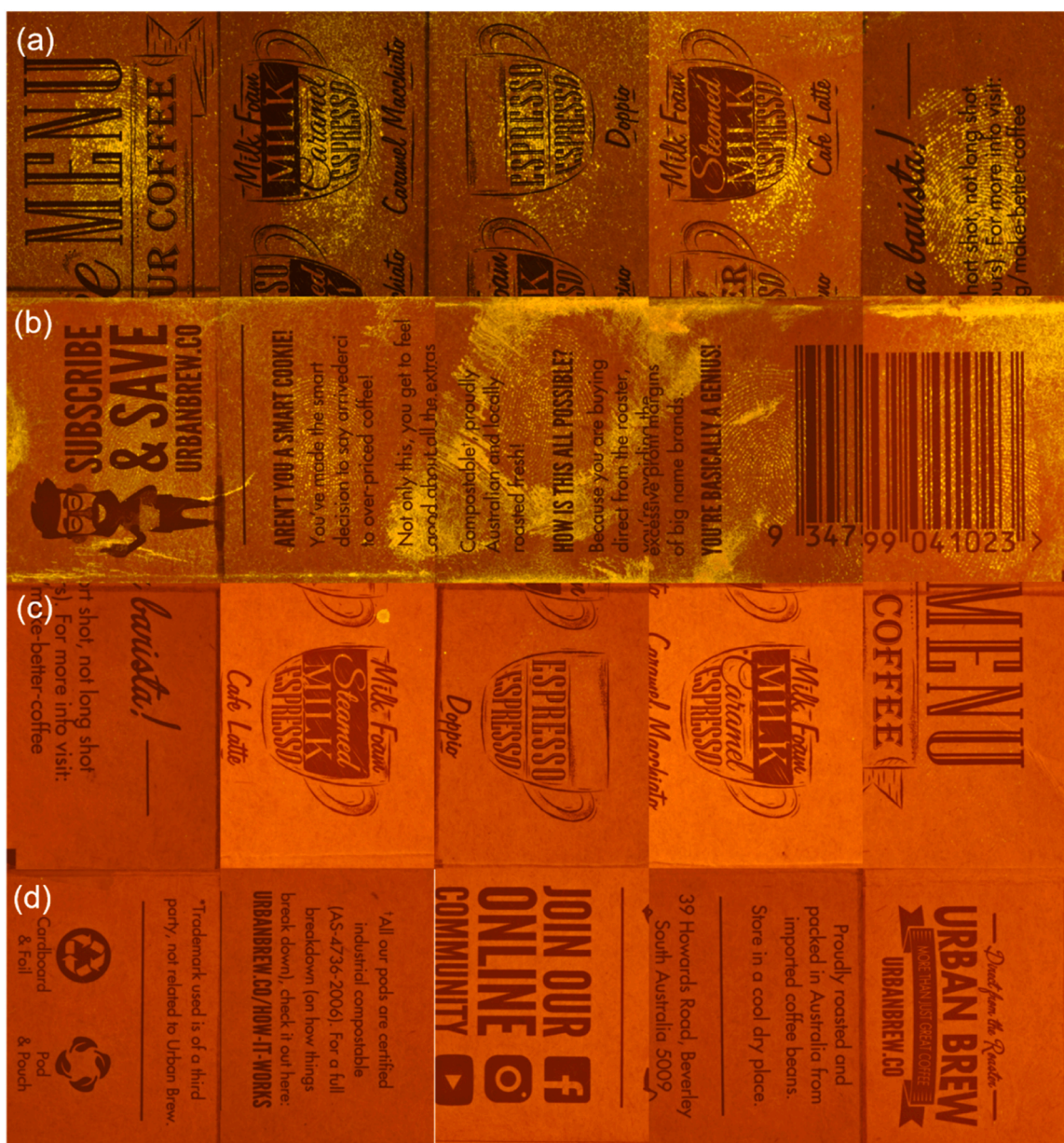
Fig. 11. Fingermarks from D3 developed on recycled cardboard packaging using the (a) petroleum ether (40–60 °C), (b) shellite, (c) kerosene and (d) white spirits formulations. Imaged using Rofin Polilight® PL500 (Rofin Australia Pty. Ltd., Australia) 505 nm light source with a Schott OG 550 nm (long pass) filter, photographic conditions were ISO 200, ½ sec shutter speed and f/11 aperture.
