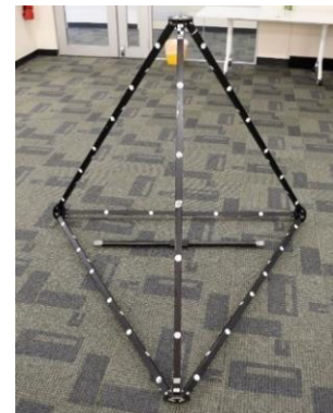
Figure 1. Proposed calibration frame assembled, with a scale bar (899.954 mm) inside it.
