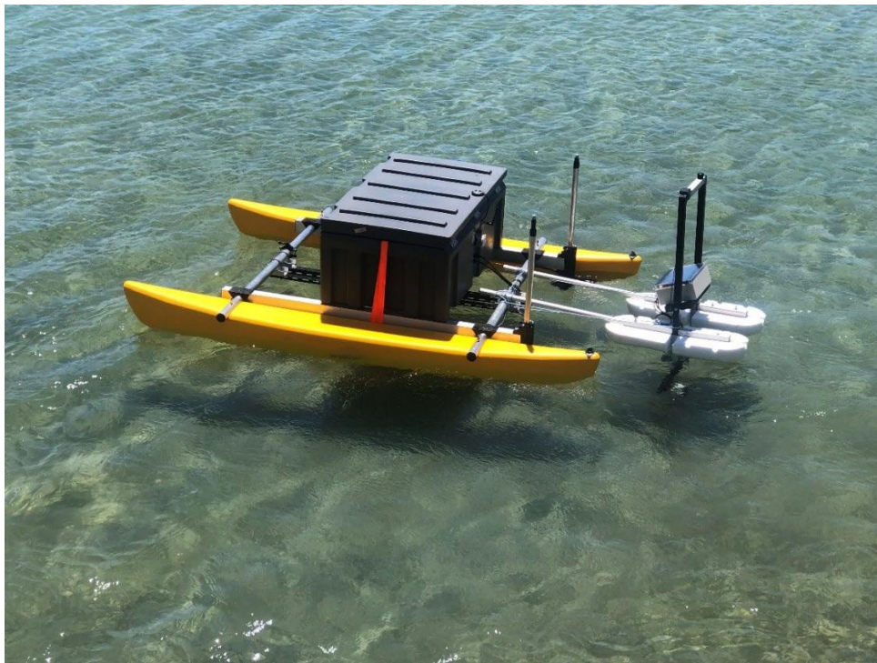
Figure 5. 1. Survey platform with logging device being pulled by an Autonomous Surface Vessel provided by Peter McKewan from PESAC Pty Ltd.
