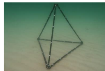
Figure 7. Proposed calibration frame underwater captured using the Canon G7X camera.
