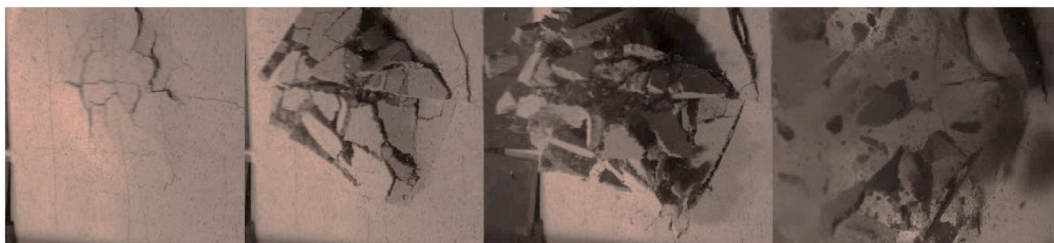
Fig. 13. Typical failure process of AAC_T50L at distal face.
