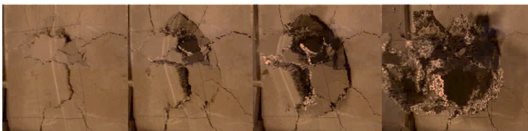
Fig. 18. Typical failure process of LGC_T50L at distal face.
