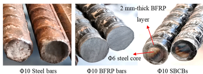
Fig. 1. Longitudinal reinforcements of the columns.
