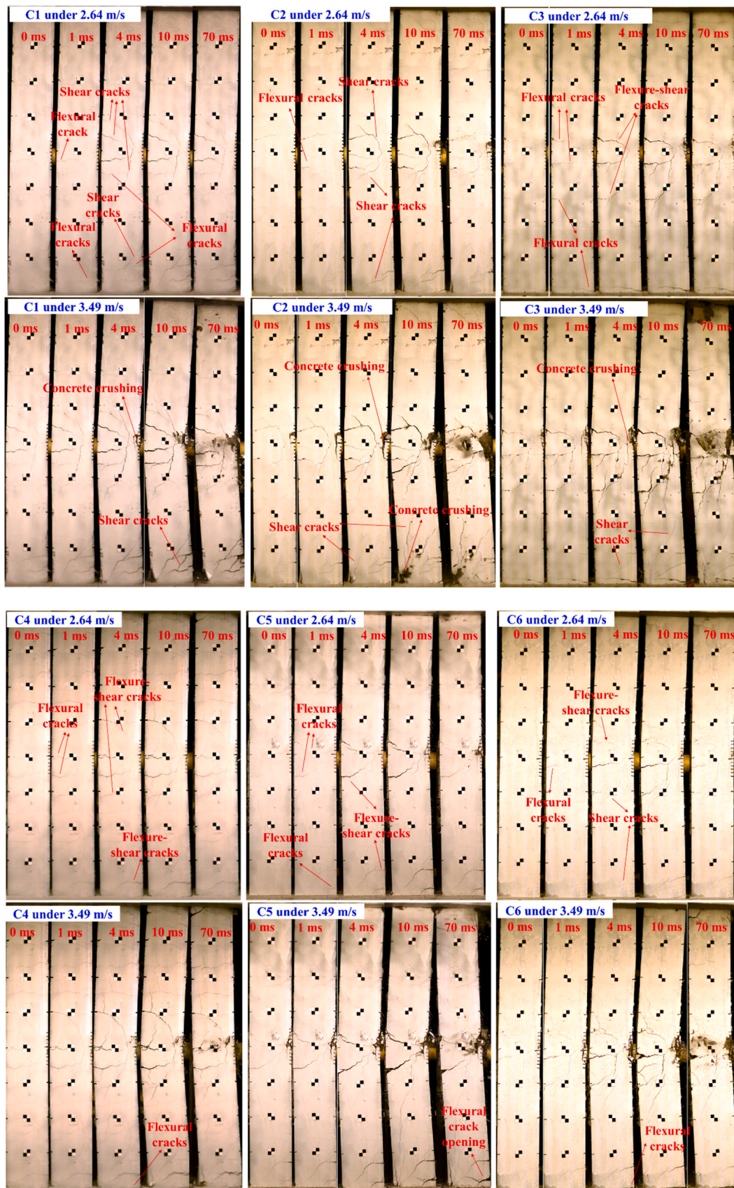
Fig. 9. Damage progression of the columns.
