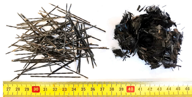
Fig. 3. Basalt macro fibres (left) and carbon fibres (right).
