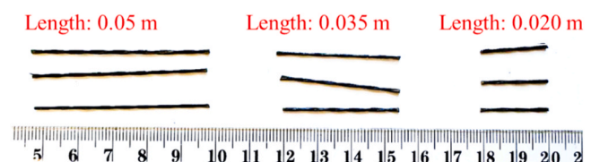
Fig. 1. Pictures of basalt macro fibres (BMFs) used in this study.
