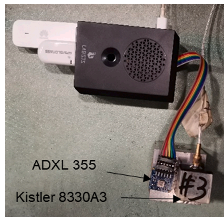
Fig. 7. Test configuration to obtain noise characteristics and sensor accuracy.
