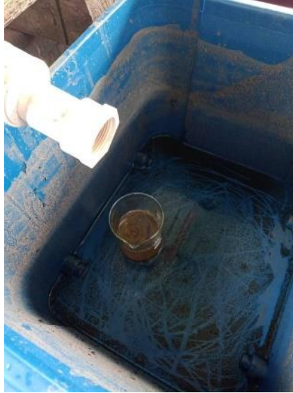
Figure 3.14: Collection of effluent from drainage pipe.
