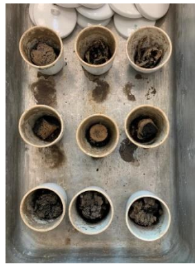
Figure 3.18: Dried sludge sample after furnace test.
