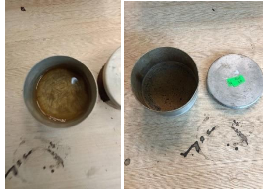
Figure 3.20: Dried effluent sample before (left) and after (right) oven test.
