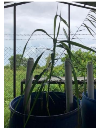
Figure 4.12: The reed bed after acclimatization.
