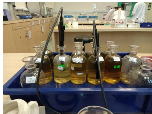
Figure 3.25: Reading and evaluating of effluent concentrations using portable multimeter with respective probes.
