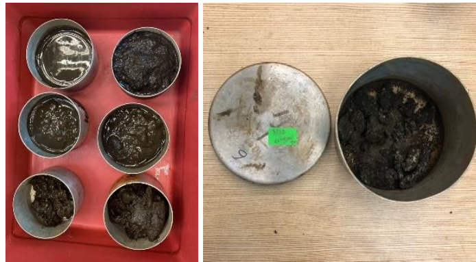
Figure 3.17: Dried sludge sample before (left) and after (right) oven test.
