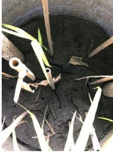
Figure 2.5: Crack occurrence on the sludge deposit layer.
