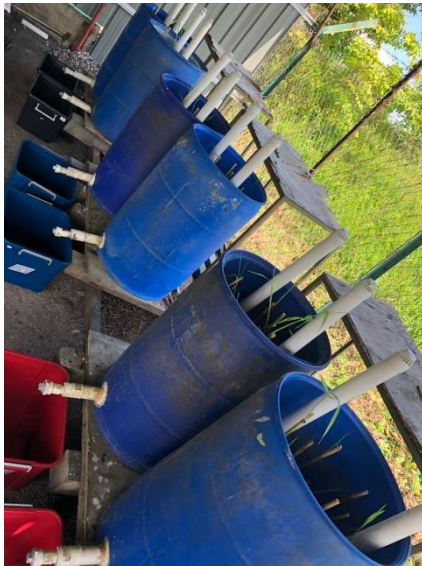
Figure 3.10: Actual experimental illustration of laboratory-scale STRBs.
