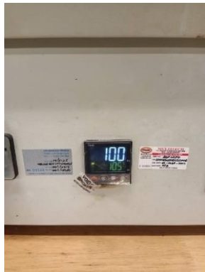
Figure 3.16: Oven with set temperature 105°C.
