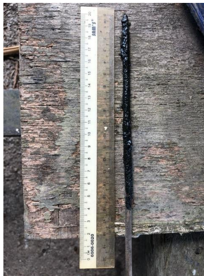
Figure 3.15: Measurement of sludge deposit thickness.
