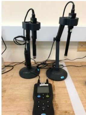
Figure 3.24: HACH HQ40d portable multimeter with IntelliCAL™ LDO101 standard luminescent / Optical dissolved oxygen (LDO) probe (left).
