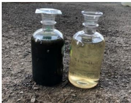
Figure 4.13: Turbidity difference between raw septage (left) and effluent (right).
