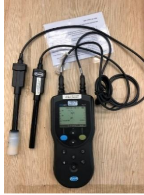
Figure 3.23: HACH HQ40d portable multimeter with pH probe (left) and NO 3 probe (right).
