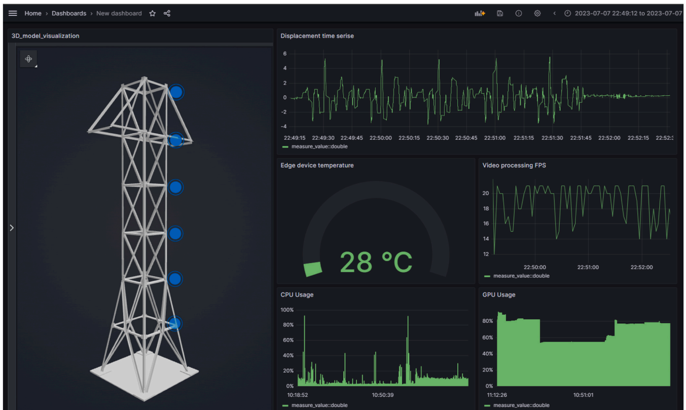
Fig. 3. Dashboard created to visualize displacement and edge device status data.
