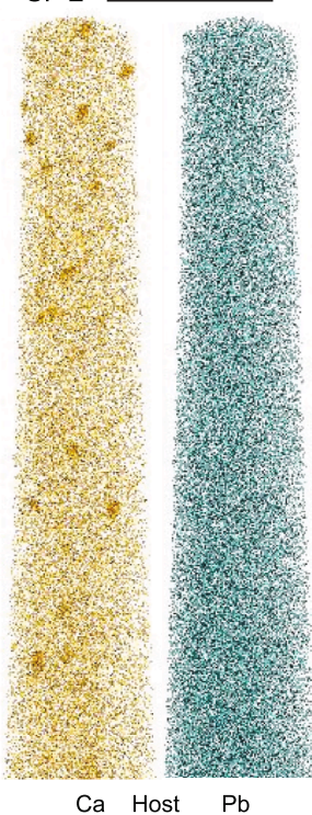
Fig. 8. Atom probe 3D reconstruction of representative specimens from Vredefort xenotime grain 14DG14 and Santa Fe grain SFx5. Each small sphere represents an atom of the indicated element. (a) Vredefort specimen V1, host xenotime from a high strain domain showing Ca and Pb* enriched clusters and a dislocation enriched in Ca, Na, Al, and OH. Cl is also distributed heterogeneously in clusters. Specimen V4 is from a neoblast and shows Ca and Pb* enriched clusters. (b) Santa Fe specimens SF1 and SF2 from host, and SF3 and SF4 from twin domains. Host and specimen show numerous Ca clusters with < 1 % Pb* clusters. Note that Pb* enriched Ca clusters are only present in specimens from the twin domain.
