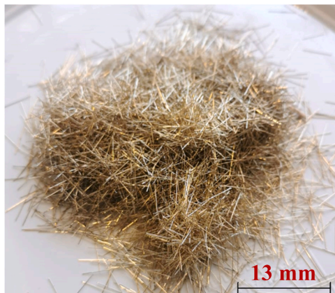
Fig. 3. Copper coated steel fibres.
