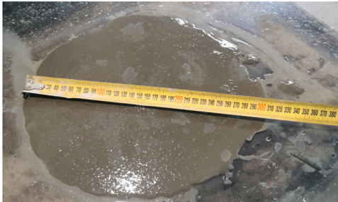
Fig. 5. Slump flow diameter of reference mix.
