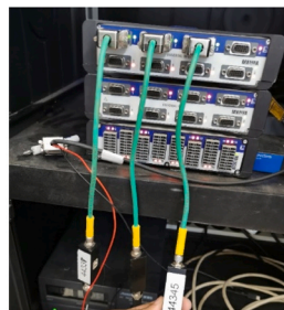
(b) HBM data logger for accelerometers
