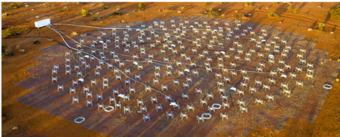
Figure 1.5: The aerial view of the EDA2. The SMART boxes are seen as the small white boxes, and the FNDH is the large white box outside the array of dipoles.
