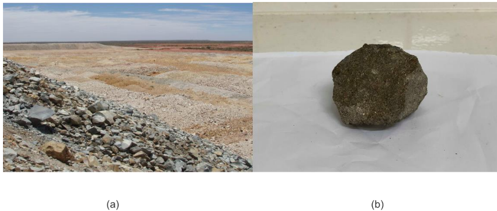
Figure 15. Nickeliferous pyrrhotite obtained from waste mine tailings in Kambalda, WA. (a) Pile of waste rocks. (b) Waste rock obtained.
