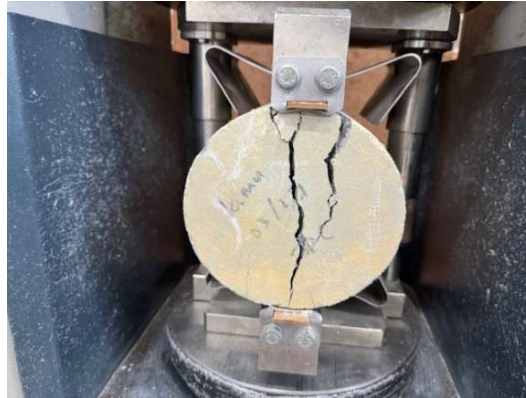
Figure 3.11: Indirect tensile strength test setup
