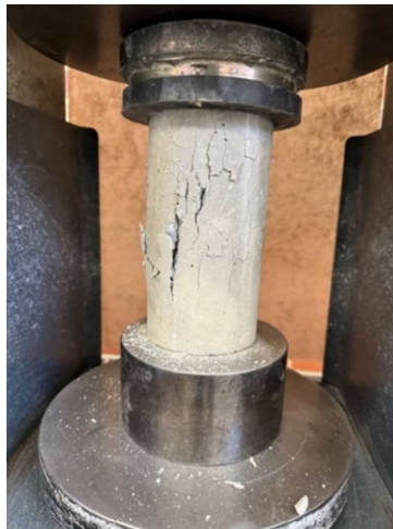
Figure 3.10: Compressive strength test setup
