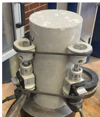
Figure 3.12: Modulus of elasticity test preparation
