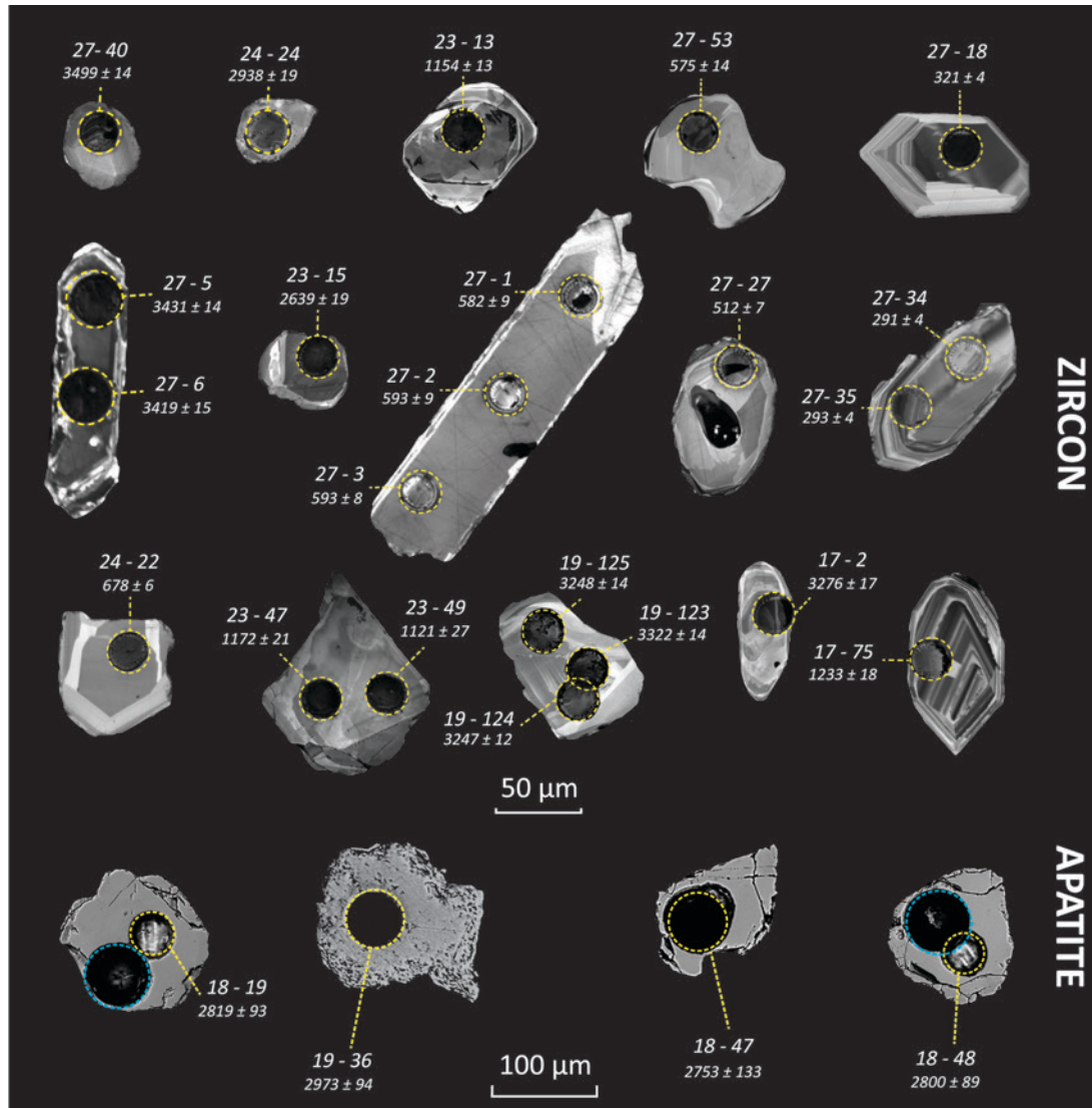
Figure 2.3. Top rows: Cathodoluminescence images of representative zircon grains showing sample and spot number, laser spot location (38 μm) and concordia age (Ma ± 2σ). Only grains ≤ 10 % discordant are shown. Bottom row: A compilation of backscatter electron images of representative apatite. The smaller spot is a 38μm U-Pb ablation, whereas the larger spot is a 50 μm ablation.
