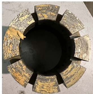
Figure 4.19: Cuttings stick on the bit face after the drilling test ( \eta = 45 s).
