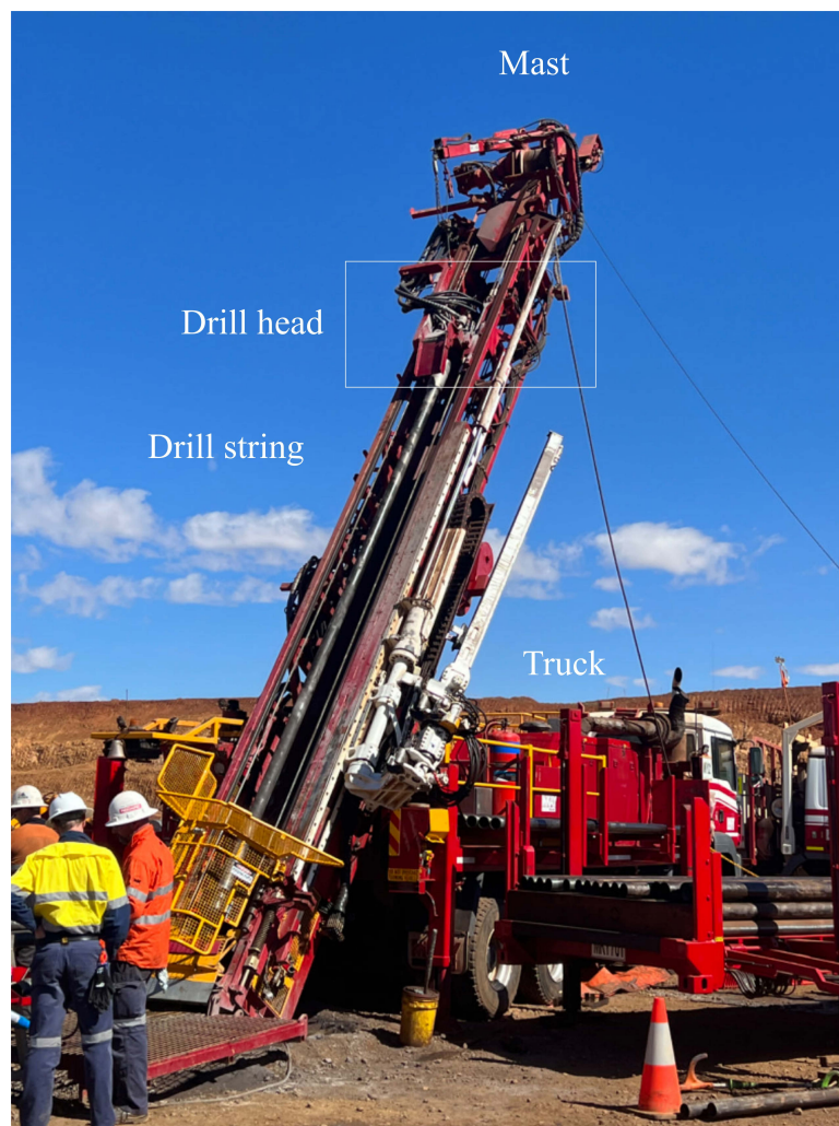
Figure 1.1: Diamond core drilling rig.
