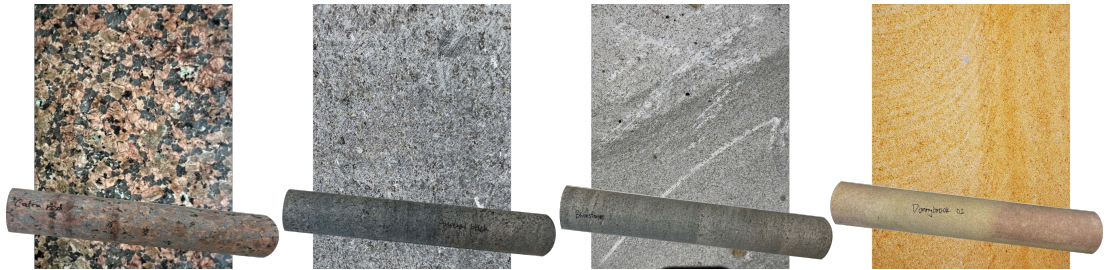
Figure 3.36: Rock sample: Donnybrook, Bluestone, Austral Black, and Calca Red (from left to right).
