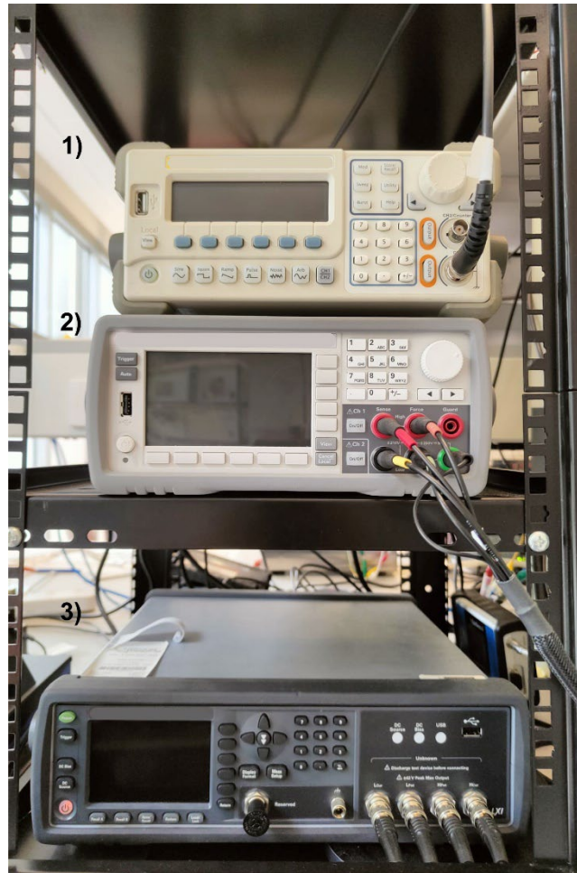
Figure S2. Instrument rack for the J–V and C–V measurements. (1) Function generator, model DG-1022, from RIGOL, (2) SMU, model B2902A, from Keysight, and (3) LCR meter, model E4980A, from Keysight.
