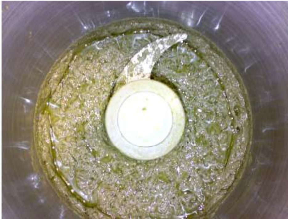
Figure 3-3: Destoned olive paste being malaxed in the Blixer 4.0 Blender as oil droplets coalesce and float to the top
