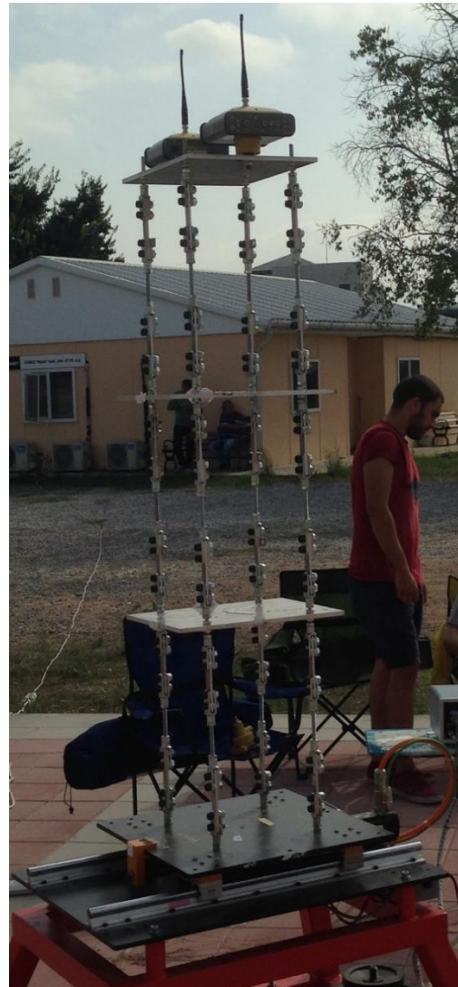
Figure 1. Small Scale Model on the shake table
