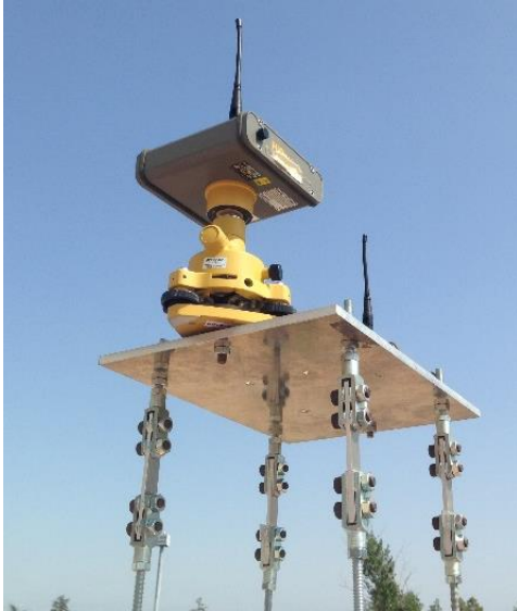
Figure 2. GNSS receivers attached on the structure model (GNSS 1 and GNSS 2 with tribrach are on right and left side, respectively)
